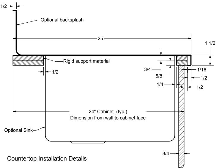
Rigid support is required under metal countertops. This support can be an existing counter top that has been properly prepared, or new plywood. The thickness of the support material should be at least 1/8" less than the height of the front edge of your counter top to ensure the support material will not be visible after the metal counter top is installed. We recommend that the support materials be field installed.
